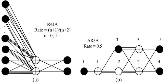
Fig. 3. The protographs of (a) an R4JA code and (b) an AR3A code.
