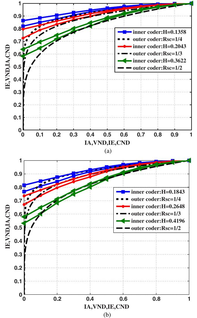
Fig. 4. PEXIT curves for inner coders are shown by solid lines, including upper-bound curves and lower-bound curves, outer coder PEXIT curves are represented by dotted lines.
