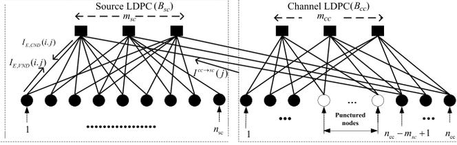
Fig. 2. Joint decoder of JSCC system with mutual information updating.
