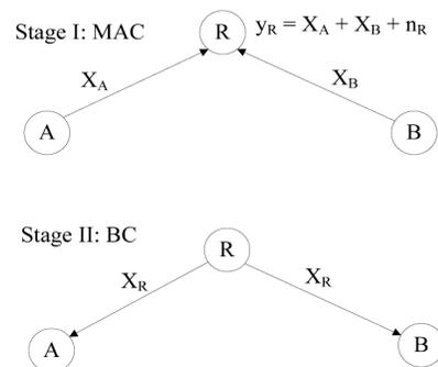
Fig. 1. Two sources A and B expect to exchange information from each other through the relay R, which comprises two stages: multiple access (MAC) and broadcast (BC).
