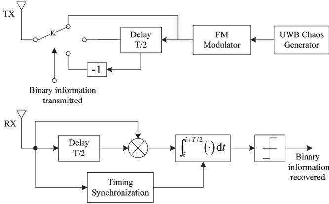
Fig. 1. Block diagrams of the FM-DCSK UWB transmitter (TX) and receiver (RX).
