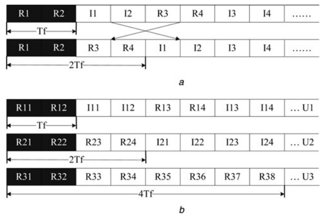
**Figure 5** Transmitted signal in the multiple-user case
