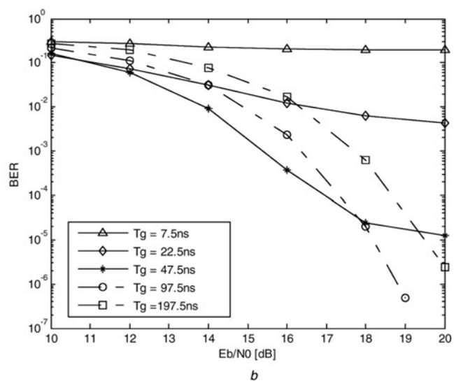
**Figure 6** Performance of the FM-DCSK UWB system with non-optimised integration interval  $T = T_f/2$  when the guard interval length  $T_g$  is 7.5, 22.5, 47.5, 97.5 and 197.5 ns
