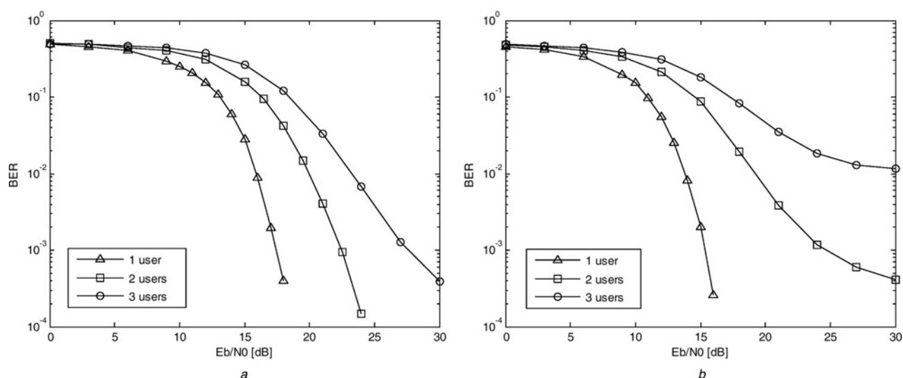
Figure 10 BER against  $E_b/N_0$  for the proposed FM-DCSK UWB system
