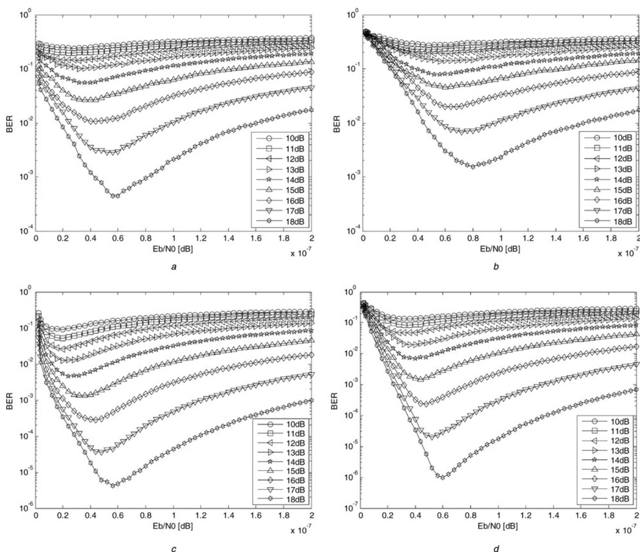
**Figure 7** BER as a function of the integration interval, as  $E_b/N_0$  increases from 10 to 18 dB in
