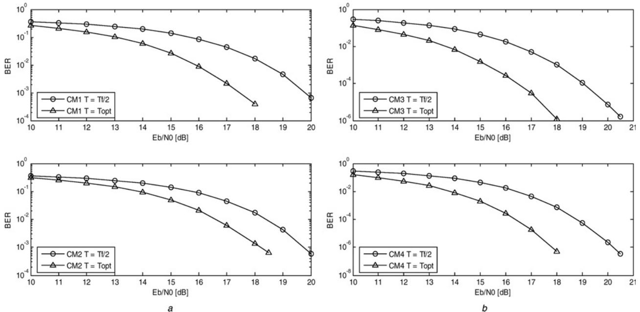
**Figure 8** Performance comparison between the original FM-DCSK UWB scheme ( $T = T_f/2$ ) and the optimisation scheme ( $T = T_{opt}$ ) with data rate at 2.5 Mbps in
