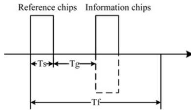
Figure 2 Signal structure of the FM-DCSK UWB system
