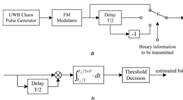
Figure 1 Block diagram of the FM-DCSK UWB system
