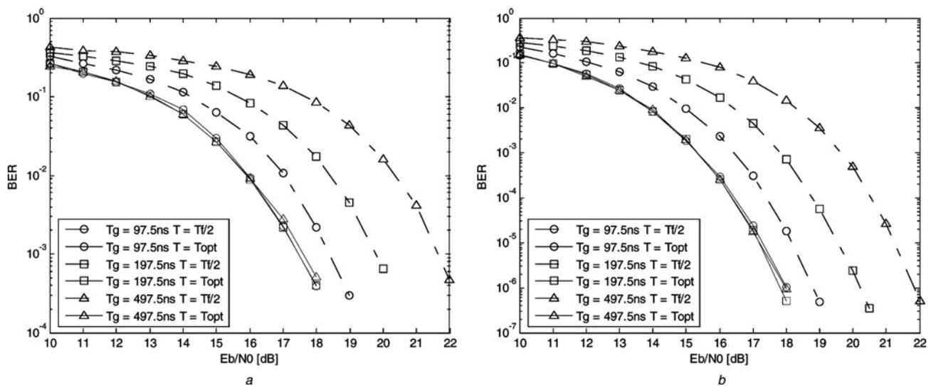
**Figure 9** Performance comparison between the original FM-DCSK UWB scheme ( $T = T_f/2$ ) and the optimisation scheme ( $T = T_{opt}$ ) with data rates at 5 Mbps ( $T_g = 97.5$  ns), 2.5 Mbps ( $T_g = 197.5$  ns) and 1 Mbps ( $T_g = 497.5$  ns) in
