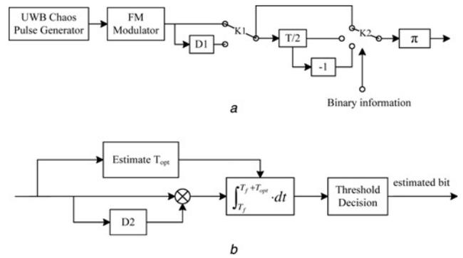
**Figure 3** Block diagram of the proposed optimisation FM-DCSK UWB system
