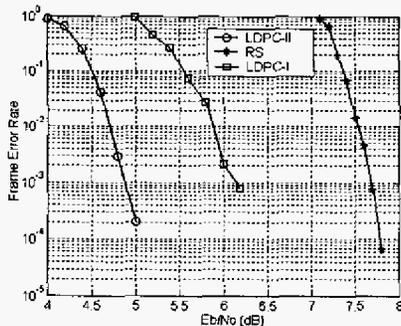
Fig. 6: Performance of non-binary LDPC codes and RS codes over noise bursts channels with burst-length 144 bits
