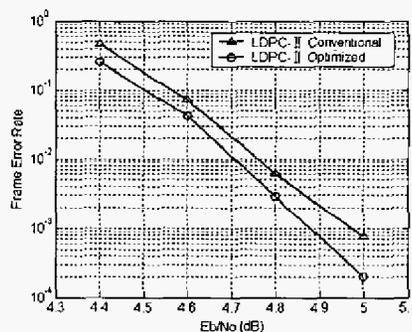
Fig. 7: Optimized encoding scheme Vs Conventional encoding scheme
