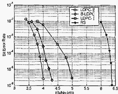
Fig. 5: Performance of LDPC codes and RS codes over AWGN channels
